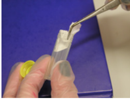
Figure 6. Odour-infused muslin was provided to the trainer in 5mL polypropylene tubes for detection of AFB.
